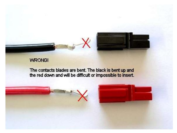
Tug slightly on the assembled connector to make sure the contacts are locked in place. If you have trouble getting the contact to lock in to the housing you may have squashed the contact wider deformed it some how. Look at the side profile of the contacts before and after crimping, you may have to bend it back straight before inserting it in to the housing.
